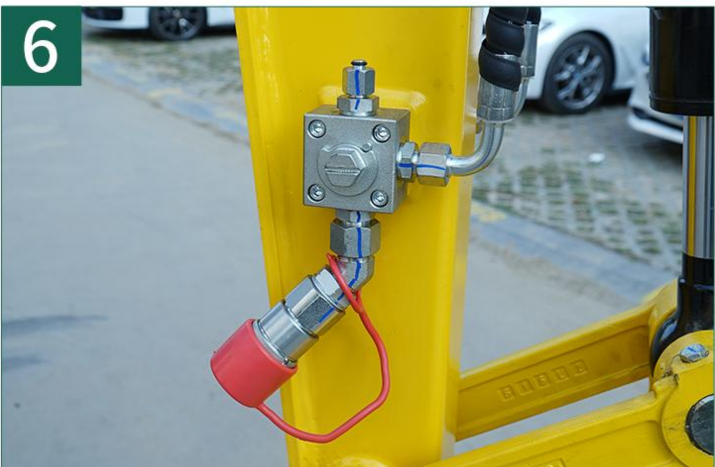
Crushing hammer shut-off valve
