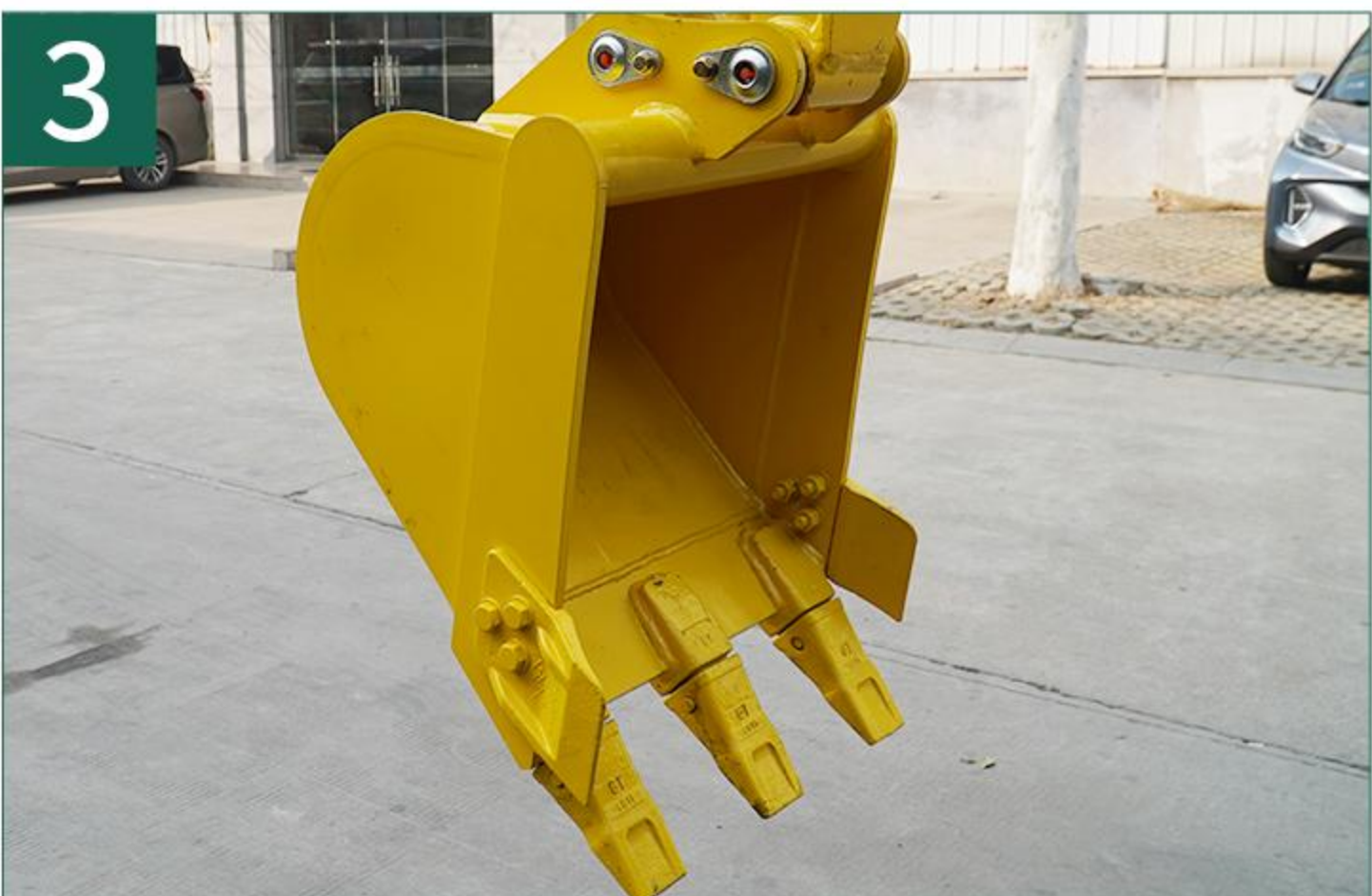
Thickened large excavation bucket
